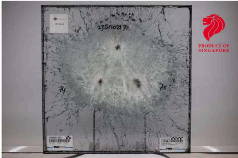
Strike Face, sample 23SA01634 after test 23MB01323
