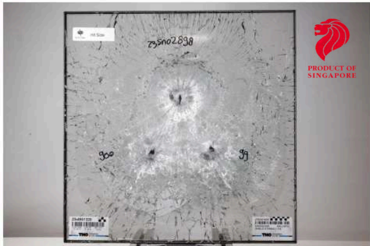
Strike Face, sample 23SA01605 after test 23MB01320
